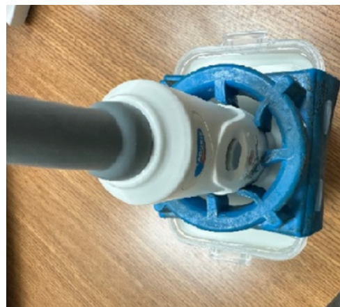
Bladder Phantom, Probe Holder and Bladder Scanner Probe
